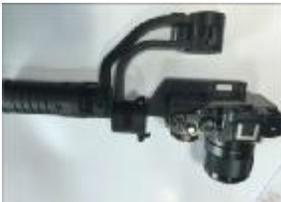
D. adjust camera YAW balance, check pic above, hold camer as above, balanced, means YAW balanced. if not, adjust YAW motor side 2 screw to move arm, then tight screw after balanced.
