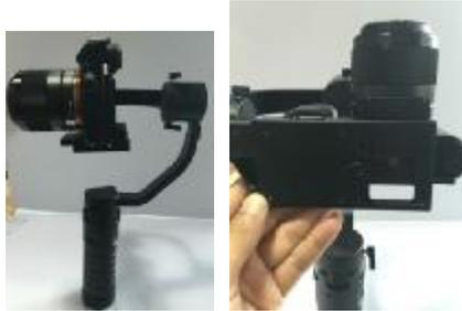
B: adjust camera front/back balance ,arm adjust , then lock pitch motor side 2 screw
