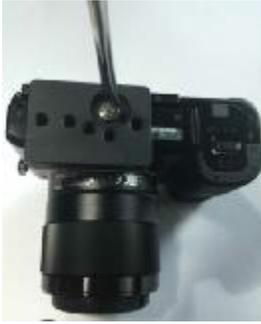
adapter plate installing
